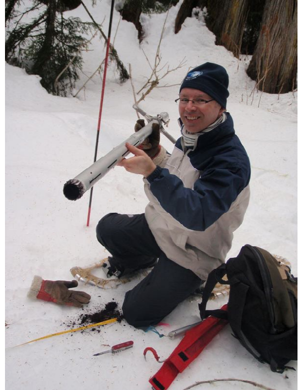
Dr. Stephen Déry extracting a snow core with a Federal Sampler in the inland rainforest, 5th March 2010.
